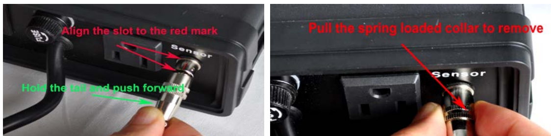
Figure 2. Maneuvers to install (left) and remove (right) the sensor.
